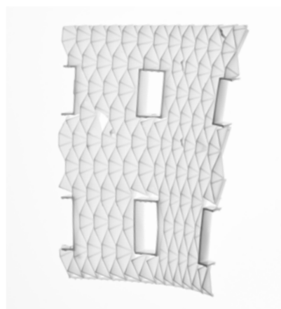
This complex facade is parametrically designed based on a sun path analysis, and would be incredibly difficult to fabricate by any other means at such a scale.
