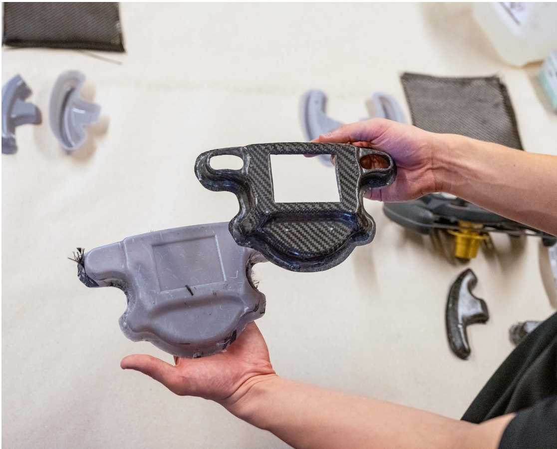
A 3D printed mold for hand laminating carbon fiber parts.
