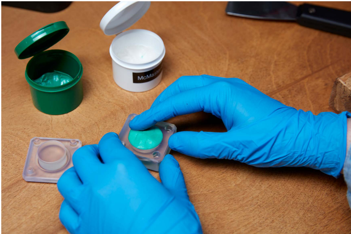
The silicone mixture being placed into the 3D printed mold.
