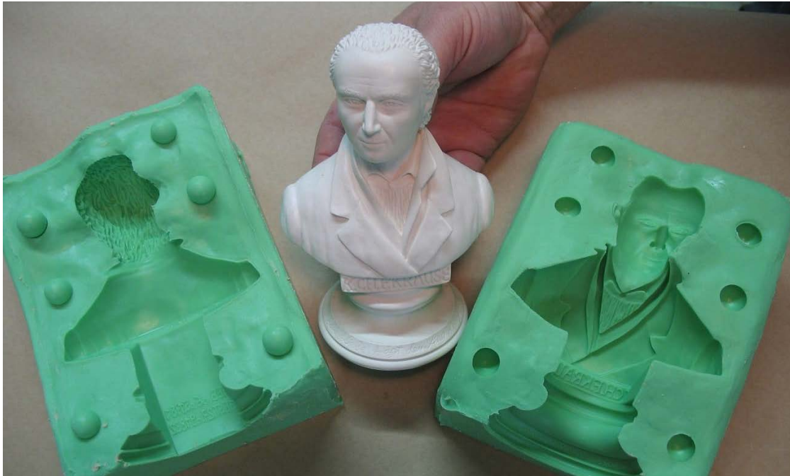
Two-piece silicone molds can reproduce any master design ( image source )
