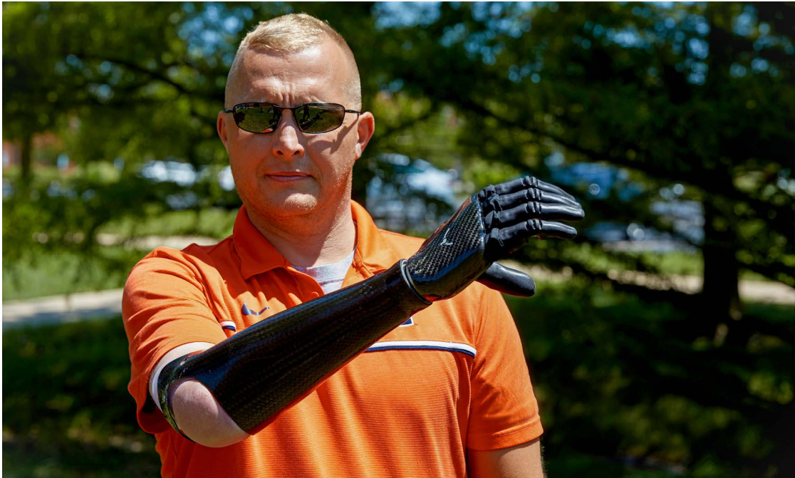
The PSYONIC Ability Hand, created with multiple 3D printing technologies, including Formlabs SLA.
