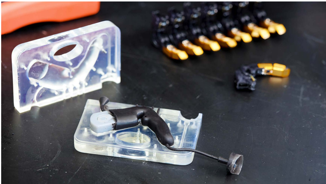
Part of the PSYONIC Ability Arm , a pioneering bionic prosthetic, is created using 3D printed molds.
