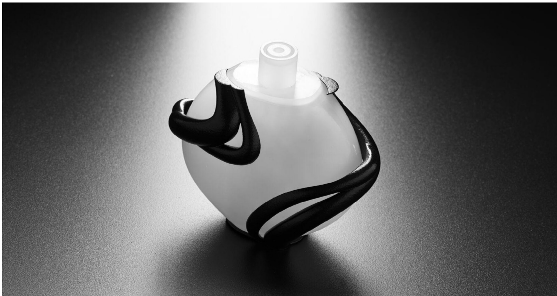
Custom perfume bottle packaging including a black wrapping feature that was printed on the Fuse Series SLS 3D printer in Nylon 11 Powder and then vapor smoothed.
