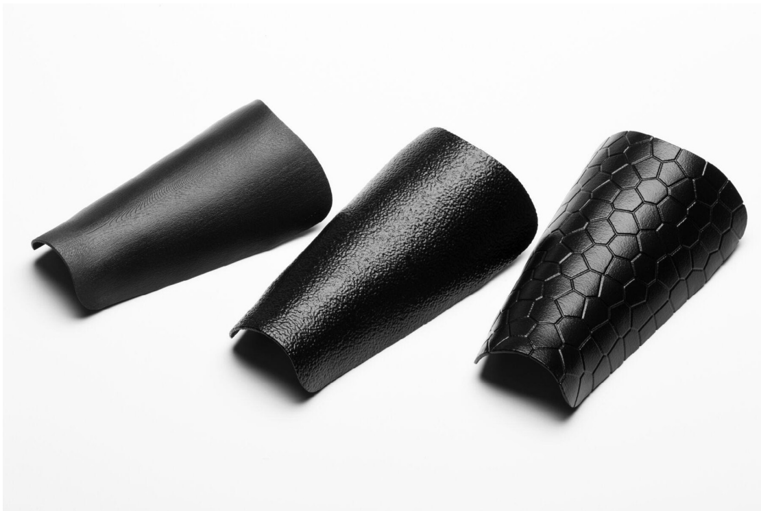
3D printed lightweight, customized shin guards are an application that benefits from reduced bacteria growth. Printed in Nylon 11 Powder and vapor smoothed.
