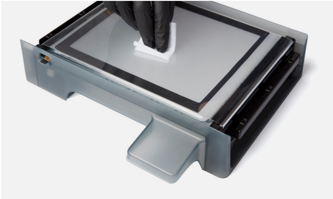
Cleaning the bottom of the tank using photographic wipes (PEC-PADs) and Isopropyl Alcohol.
