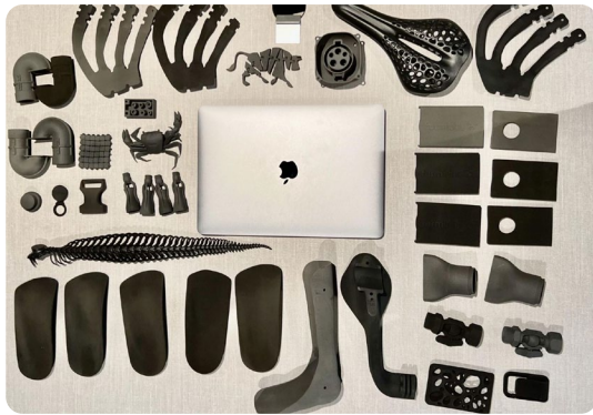
This photo represents 1kg of parts (laptop included for scale representation). If you needed to print this amount each day, you'd be on target for about 240 kg of printed powder each year.
