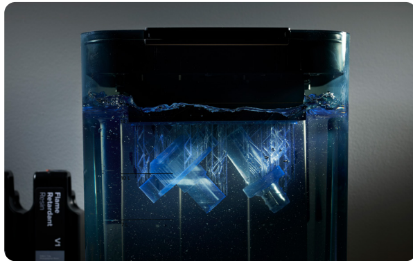
Formlabs' second-generation Form Wash has improved agitation and a larger volume to make cleaning parts easier than ever.
