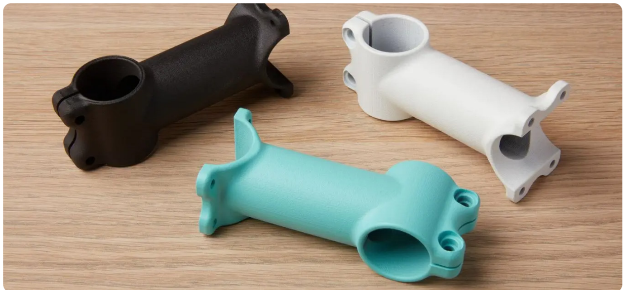
Coatings like Cerakote can reinforce SLA 3D printed parts and make them stronger, more durable, and more aesthetically pleasing.
