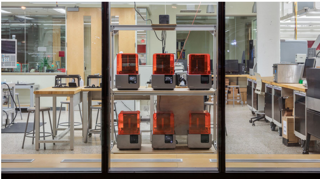
Formlabs desktop SLA units are easily stacked into shelving units and can fit into typical office spaces, like the one seen here. Adjacent tables are perfect for post-processing and finishing work.
