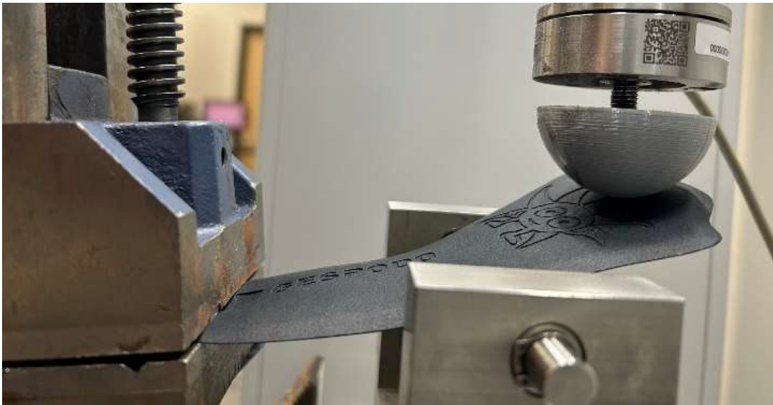
Testing setup for the Ross Flex Test indicating the position of the sample and the location of the load application
