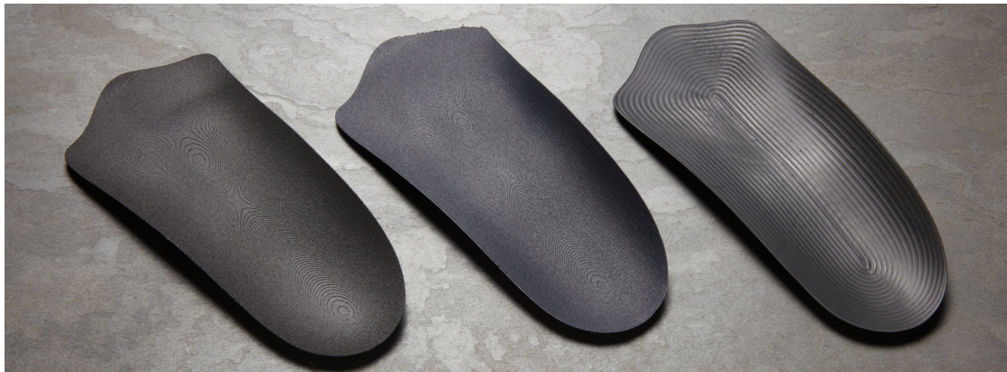
Rigid insole shell samples used in external mechanical property testing. From left to right: Formlabs Nylon 11 Powder, HP PA 11, CNC machined polypropylene
