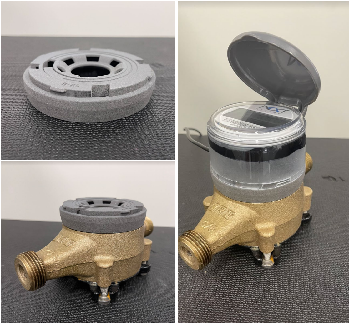
The mounting ring 3D printed in Nylon 11 with Fuse 1 (top left), fitted onto a unique water meter (bottom left), and assembled with the water meter register in clear casing (right).
