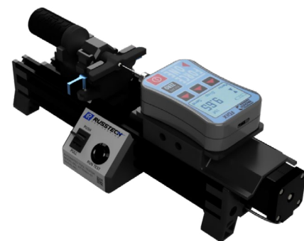
The Automated Tool Tester is driven by a stepper motor, regulated by a custom control board to regulate the cycle speed. The body is made from extruded aluminum, while the feet and various fixtures and brackets are 3D printed in Nylon 12.
