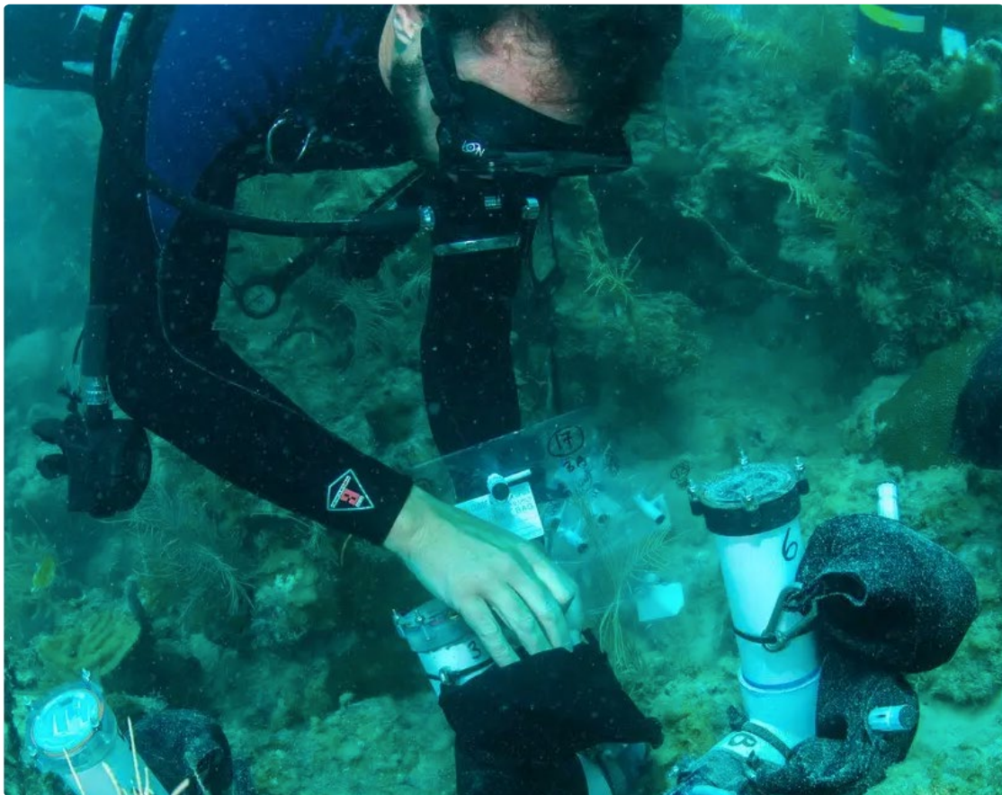
The subsurface automated samples , developed by the National Oceanic and Atmospheric Administration (NOAA), have SLA 3D printed end-caps, sample cartridges, and internal armatures. The parts are watertight and are left underwater for months for coral reef research and monitoring. (image courtesy of NOAA)
